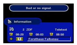
"Bad or no signal" indicates that there is a fault in the reception system or in the receiver settings or the transponder is not transmitting. Instead of the I the channel identifier shows a satellite antenna together with the message "bad or no signal". Check the SAT-IF connection and the LNB configuration. As an aid, refer to the list of
